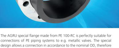
connections of PE piping systems to e.g. metallic valves. The special design allows a connection in accordance to the nominal OD, therefore the valve can be designed smaller. The dead space between the special flange and the valve is reduced, thus flow characteristics are improved which leads to a reduction of deposits and operating costs.
